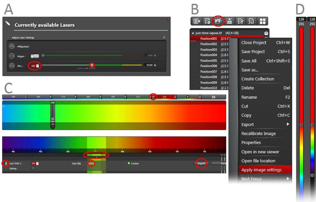
Figure 5A: Various parts of LAS X's user interface. (A) 'Laser Config'. (B) 'Open Projects'. (C) 'Acquire'. (D) Bit-depth slide bar.
